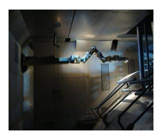
We employ automation and robotics to achieve faster, cheaper, and safer inspections. Robotics are used to lessen the dose received by our technicians while performing nuclear inspections.
